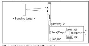
X1: Load connection for NPN output **X2**: Load connection for PNP output
