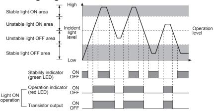
\*\*The waveforms of "Operation indicator" and "Transistor output" are for Light ON operation.
